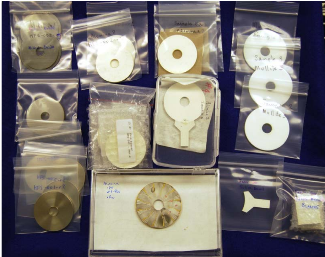
Figure 27. Ceramic and Metallic Test Samples for Robustness Testing.
