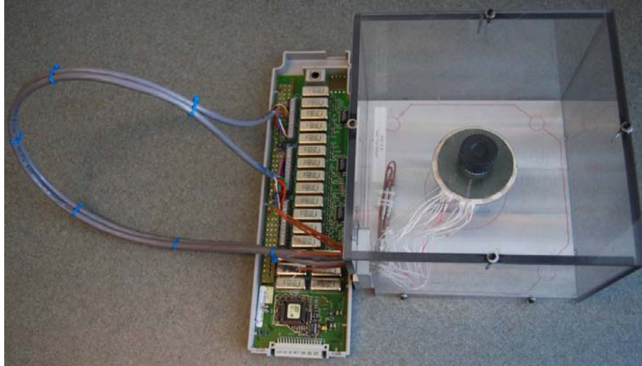
Figure 39. Completed Sensor & Spacer Assembly Wired to Agilent Multiplexer Card.
