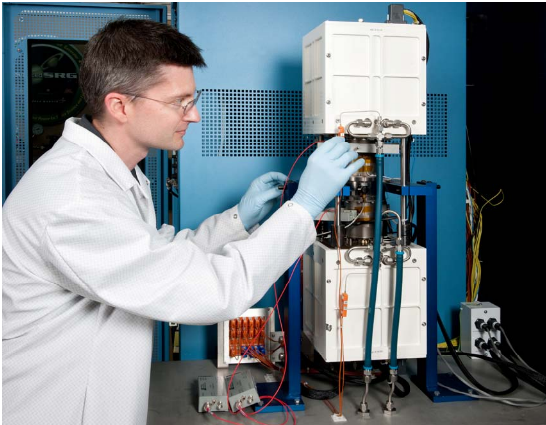
Figure 2. Test Setup for Advanced Stirling Convertor Engineering Unit (ASC-E).
