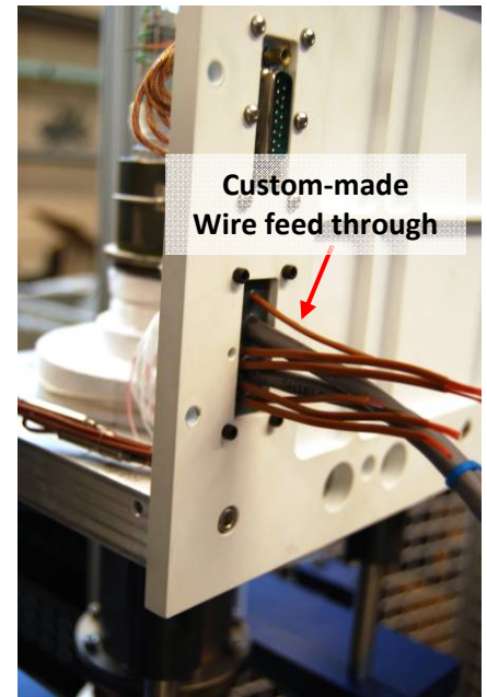
(D) Exterior view of custom-made wire feed through.
