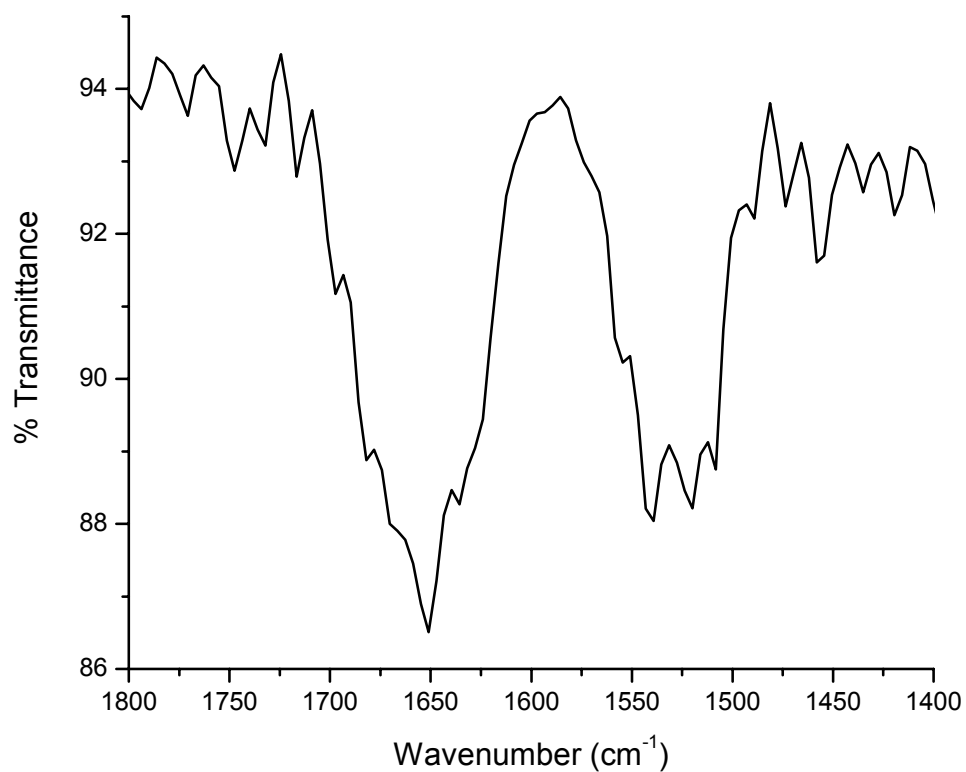
Figure 2.3: The infrared spectra of iNOSoxy/DDAB dried film, which had been denatured by heating in aqueous solution at 70°C.
