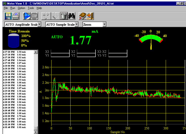
Figure 20 Anodization current density acquisition using Meterview 1.0
