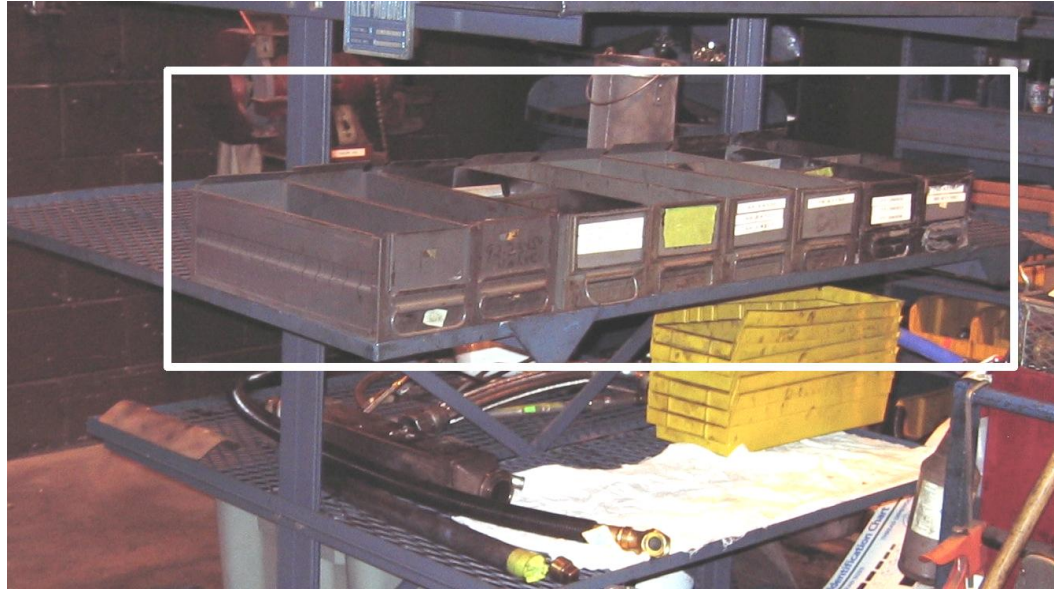
Figure 13: Special bolts bins ( poka-yoke device)
