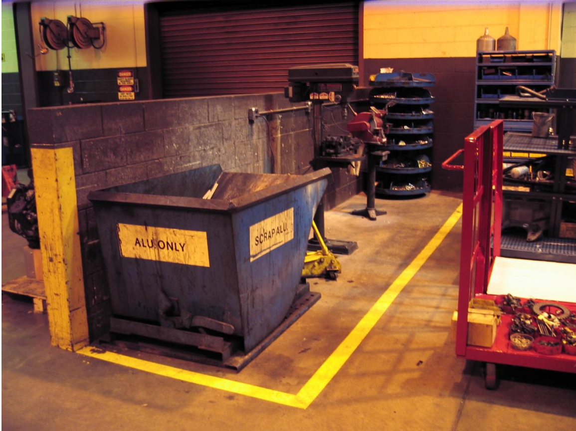
Figure 10: Portion of Engine rebuild area after 5S
