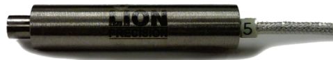
Figure 36: Lion Precision capacitance probe model C23-C applied as an additional vibration sensor outside of the spindle housing.
