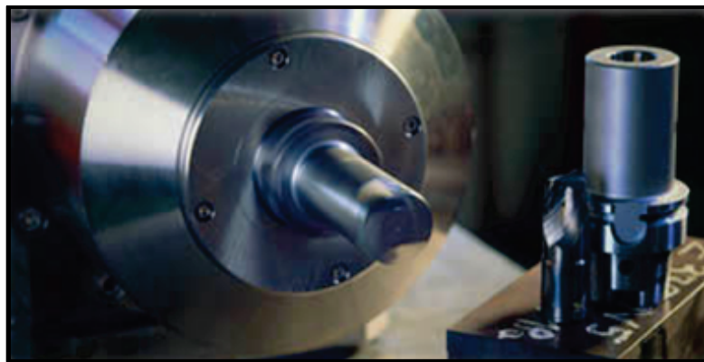
Figure 11: S2M magnetic bearing machining spindle [38].
