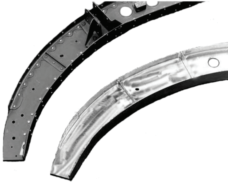
Figure 2: Airframe component, standard (top) and monolithic (bottom) construction [10].
