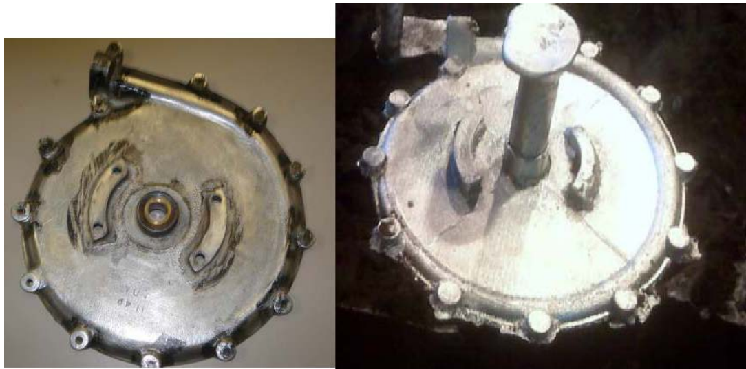
Figure 17 Comparison of the Sample Part and Reverse Engineered Part
