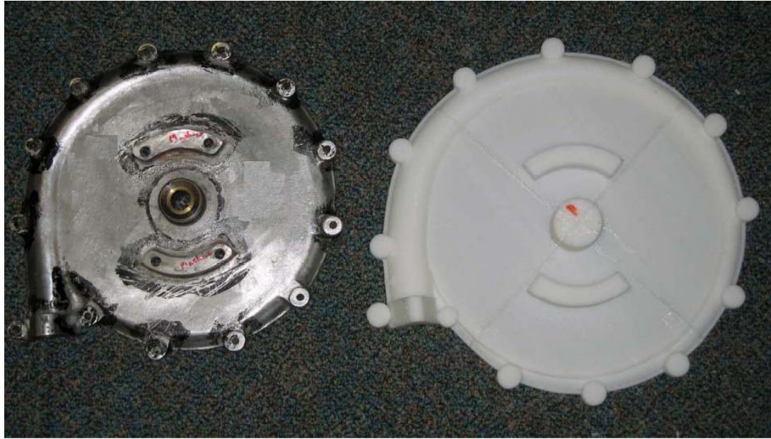
Figure 14 Comparison of sample part and ABS pattern
