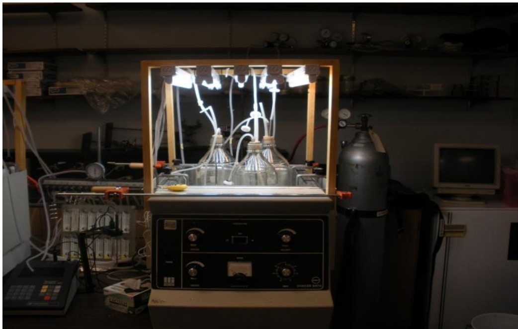
Figure 3.1. Culturing Scenedesmus dimorphus in water bath shaker system.
