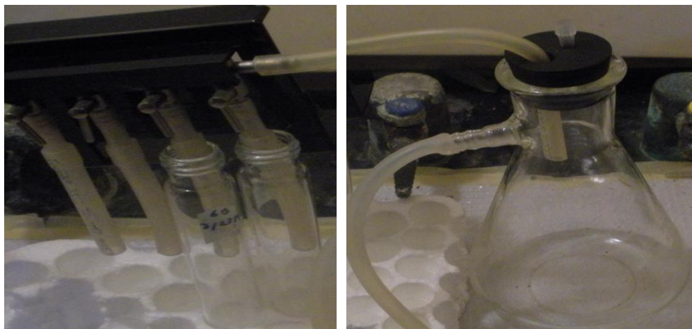
Figure 3.3. Vacuum and aspirator systems.
