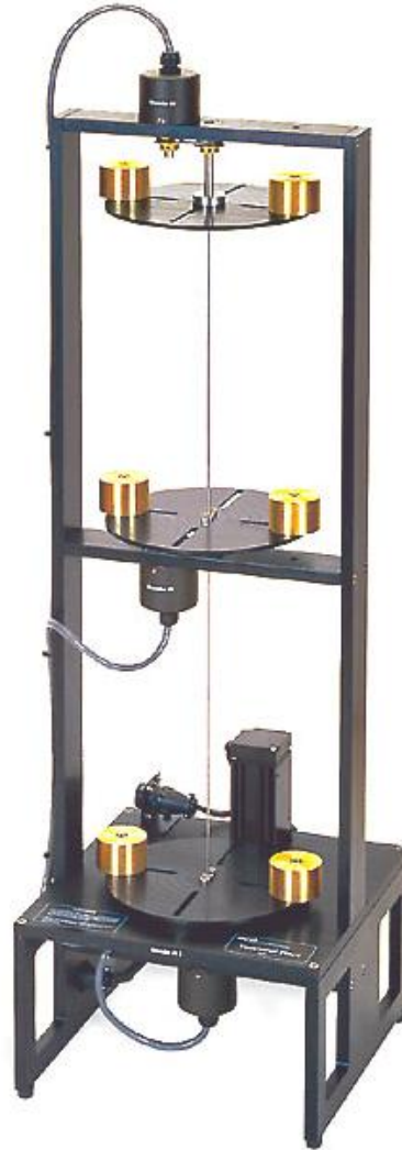
Figure 1: Photo of torsional plant
