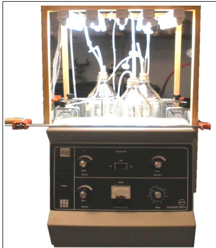
Fig2.3 Shaker water bath and lighting configuration.
