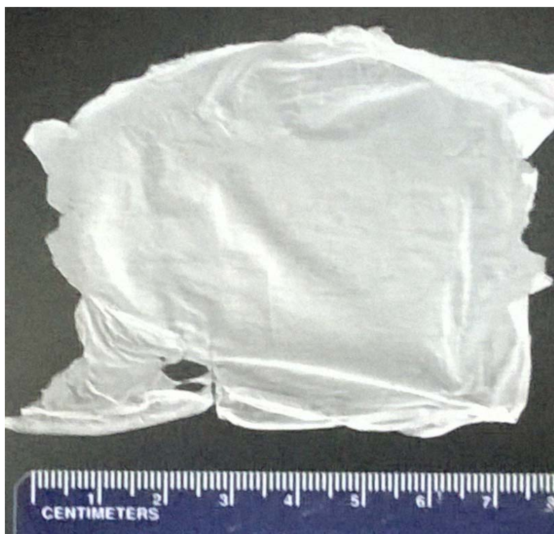
Figure 36: A photograph of a section of PVA scaffold retrieved from the large mandrel immediately after electrospinning. Electrospinning conditions: Air-gap distance: 15 cm, Potential: 15 kV, Electrospinning emulsion ratio (v/v): 20:1 (Polymer mixture : iNOSoxy containing buffer), Flow rate 1 ml/hr.
