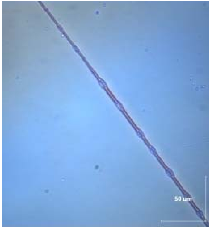
Figure 37: Optical microscopic images of PCL microfibers stained with Sudan IV.
