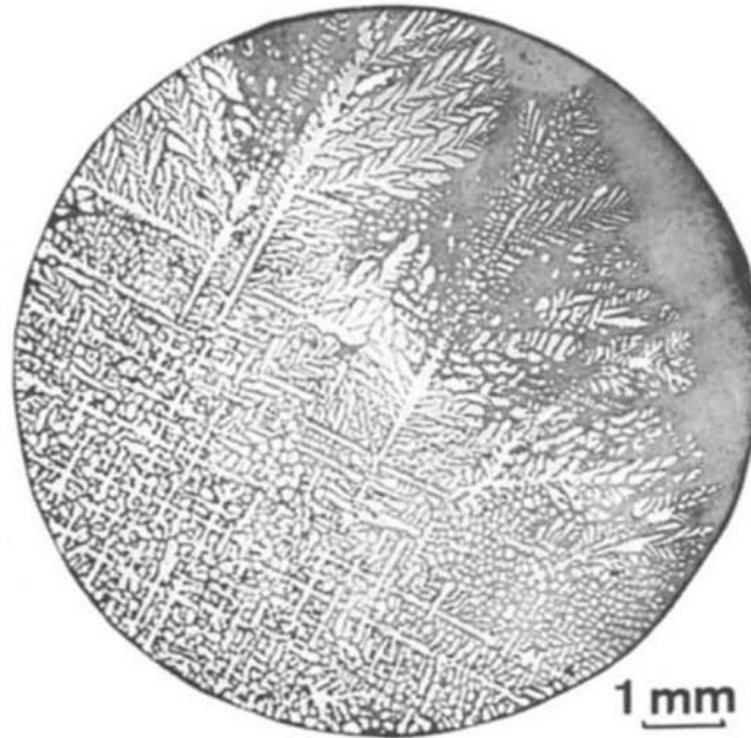
Figure 5: Image of transverse slice of an Al-26.5 wt% Cu copper alloy, grown with 30 \text{ K cm}^{-1} thermal gradient at 4.2 \mu\text{m s}^{-1} [12]. This depicts an example of transverse phase macrosegregation.
