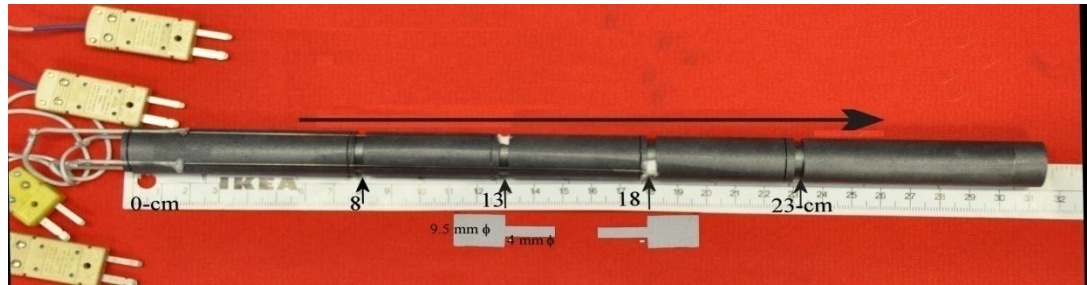
Figure 8: Image of typical graphite crucible used for solidification. 30 cm long and 1.9 cm outside diameter with 13 cm long by 9.5 mm diameter cavity on both ends, and a 5 cm long by 3.2 mm diameter cavity in the center. Thermocouples ID# TC1, TC2, TC3, and TC4 mounted at 8, 13, 18, and 23 cm respectively from the 'cold-end' or bottom.
