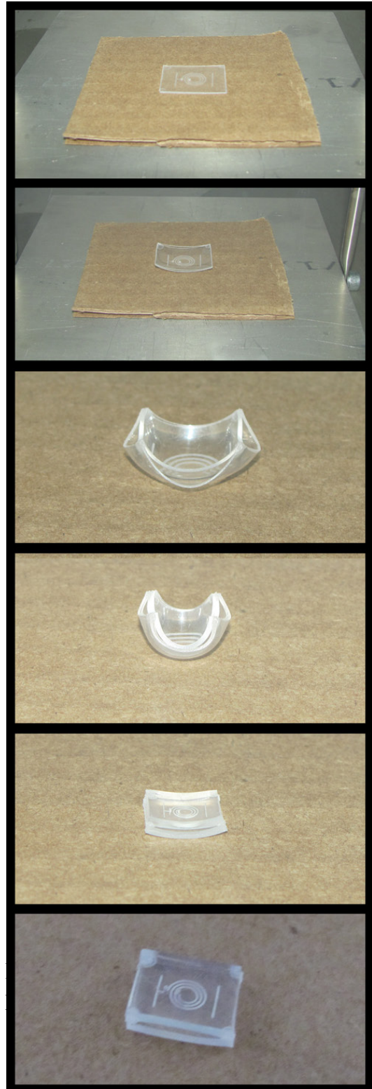
Figure 8: Milled and adhered thermoplastic sheets shrinking in oven.
