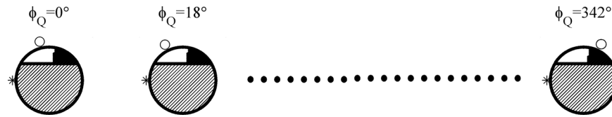
Fig. 14 Crack breathing at subsequent phases of the exciting torque; 25% crack; f_Q = 60 Hz; \vartheta = 90 deg
