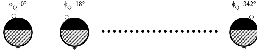
Fig. 17 Crack breathing at subsequent phases of the exciting torque; 40% crack; f_Q = 80 Hz; \vartheta = 180 deg
