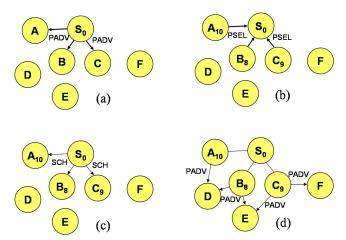
Figure 4 Three-way handshaking in MOSS. (PSEL collision and PSEL capturing can happen in (b). Multiple PADVs and PADV collision can happen in (d).)
