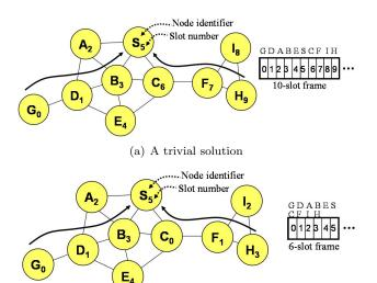
(b) A solution based on two-hop graph coloring algorithm
