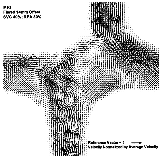
FIGURE 4. Magnetic resonance phase velocity mapping vector plot of flow in the flared 14 mm (1 caval diameter) offset TCPC model. The SVC:IVC flow ratio was 40:60 with 50% of the total flow to the RPA.
