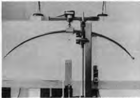
A yew longbow being tested for drawing strength. It cracked at a pressure of 24.8 kg.
