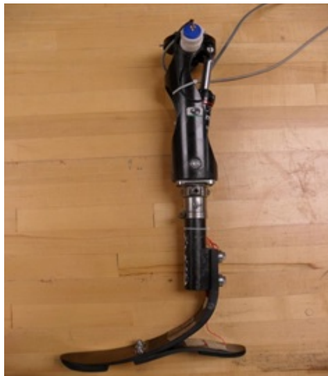
Figure 1: An Ossur Mauch knee. This prosthesis acts as a variable damper to restore proper gait during swing phase.
