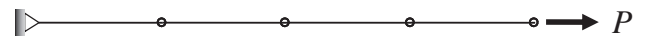
Fig. 3. Optimized design for the simple column example under tensile load P for both 10% variability and 20% variability in location of node A.
