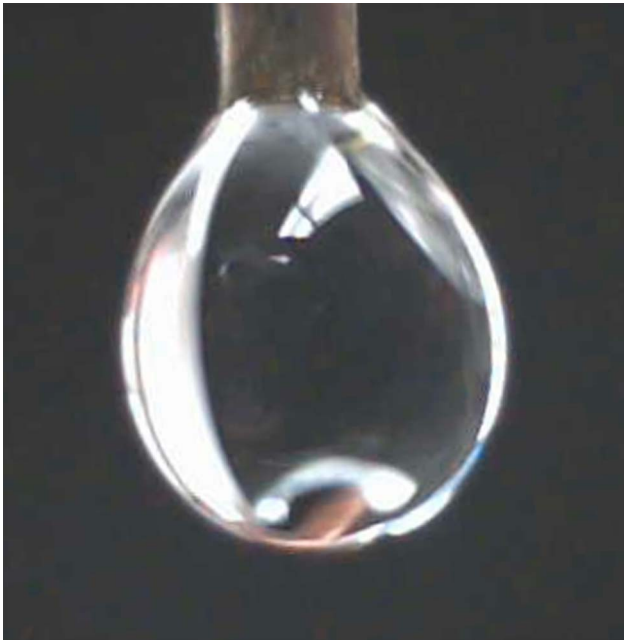
Fig. 8. (Color online) Photograph of pendant droplet. The image has been cropped slightly. The droplet is viewed from the forward (i.e., \theta = 0 ) direction; the laser beam creating the caustic will be reflected from the droplet at its upper right.
