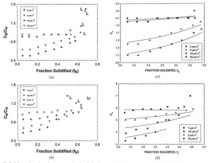
Fig. 2—Influence of growth speed on macrosegregation along the length of directionally solidified Pb-Sb alloys ( $G_l = 140 \text{ K cm}^{-1}$ ): (a) Pb-2.2 wt pct Sb and (b) Pb-5.8 wt pct Sb.
