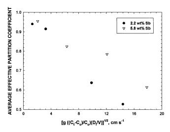
Fig. 6—Correlation between the extent of longitudinal macrosegregation as indicated by the effective partition coefficient and the parameter  $[g(C_t - C_o)D_t/VC_o]^{1/2}$ , which represents the extent of convection caused by the build up of low density solute at the tips of cellular/dendritic arrays during directional solidification of hypoeutectic Pb-Sb alloys.
