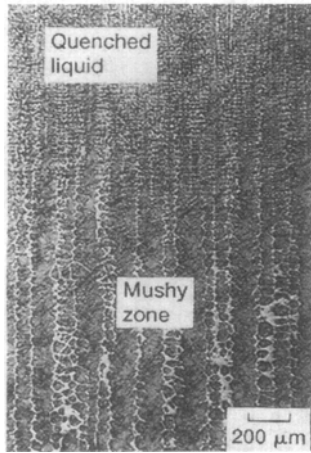
(a) Longitudinal (parallel to the growth direction at quenched liquid-solid interface).
