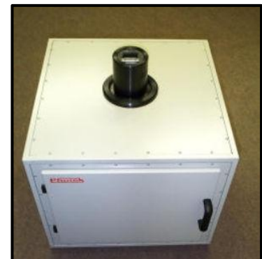
Figure 17 Photek camera (black) attached to a DB2 darkbox to prevent the interference of rogue photons. (from [FR9])
