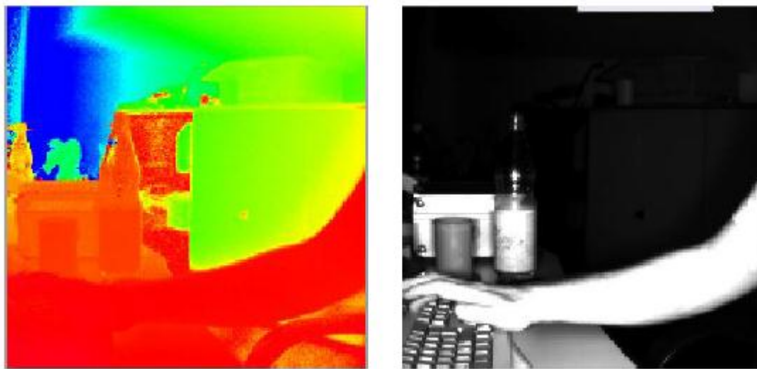
Figure 3: Time-of-Flight Images: On the left is a distance image. Here a color scale is used to display distances with close objects labeled in red and distant objects labeled in blue. On the right is an image which displays the intensity of the infrared light reflected back to the camera. This is similar but not identical to a conventional black and white image. This figure is adapted from Reference 14.
