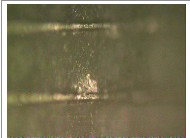
Figure 12. Metal Deposited on Insulator Surface
