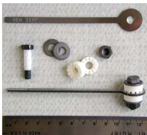
Figure 1: Multiple Crevice Assembly (MCA), bottom. It shows the lollipop-like specimen (top), titanium grade two bolt (Teflon wrapped for electrical insulation), washers nut and ceramic washers
