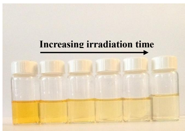
Figure 15. Decolourization of MO with irradiation time. Aliquotes taken every 2 hours,
