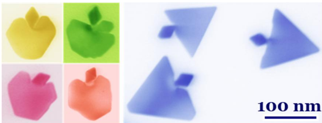
Figure 1.5. Coloured TEM images of apple and fish shaped nanoparticles prepared using the procedure developed in Ref. 37.
