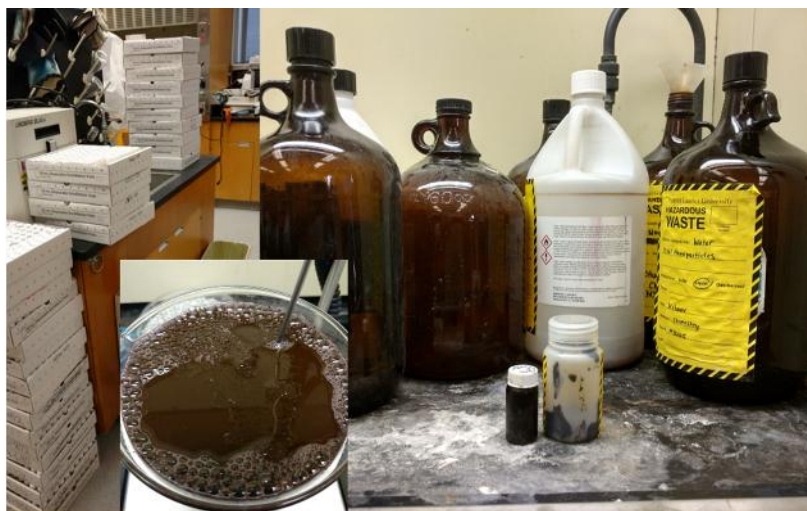
Figure 7.1. Waste disposal procedure from left to right: from vials to beaker for evaporation (or re-purposed solvent bottles), to NP sludge.
