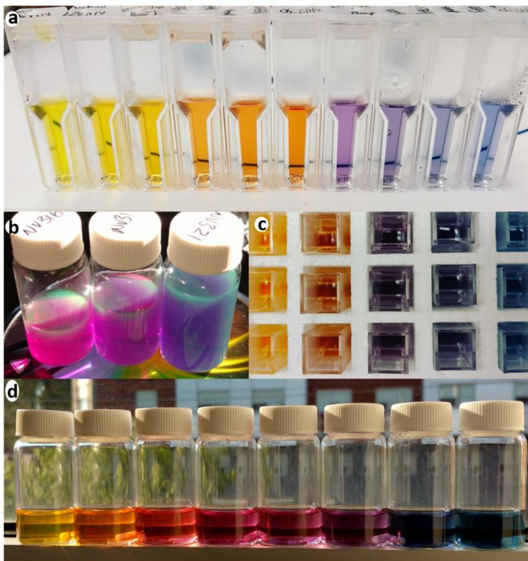
Figure 1.3. Different colours of NP dispersions attained in my research to display several “nanorainbows”, e.g. silver (with and without gold coating) nanoparticles of different sizes and shapes. a) and c) demonstrating colour changes from SPR testing of silver decahedra (with and without gold-coating) upon exposure to halides, thiols, and amines, b) silver decahedra and platelets of varying sizes, d) silver platelets of increasing size from right to left. Photographs from N. Ritter personal library of scientific images.
