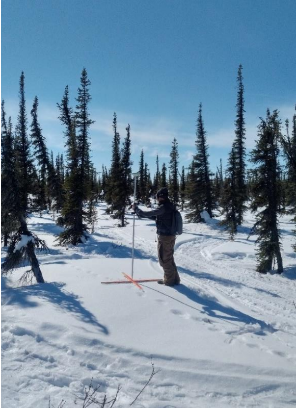
Appendix 3: Ground control point (left) marker for correcting UAS georeferencing in SfM software Postflight Terra 3D (now Pix4D). B. Walker tagging GCP using Leica GNSS RTK rover (right). GCPs were resurveyed for each UAS flight.
