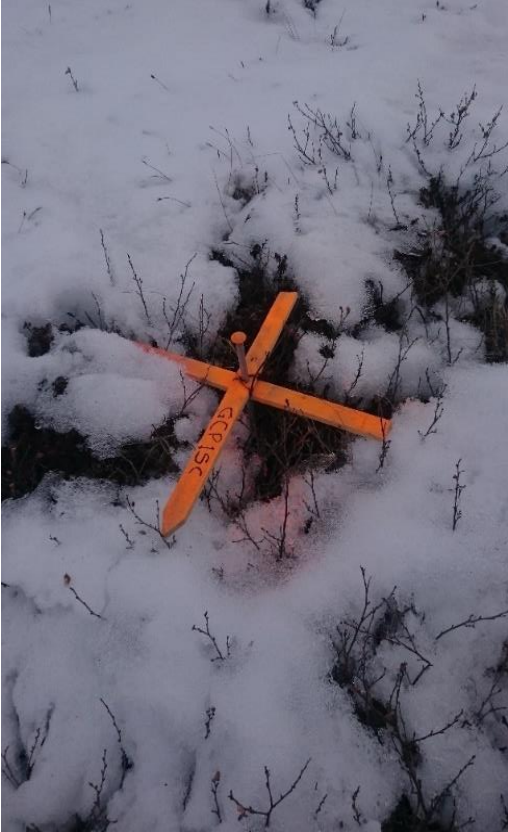
Appendix 3: Ground control point (left) marker for correcting UAS georeferencing in SfM software Postflight Terra 3D (now Pix4D). B. Walker tagging GCP using Leica GNSS RTK rover (right). GCPs were resurveyed for each UAS flight.
