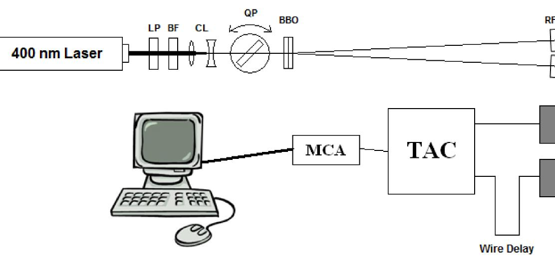
**<u>Figure #1</u>**: Theoretical diagram of experimental set-up. (LP=Laser Polarizer, BF=Blue Filter, CL=Collimating Lenses, QP=Quartz Plate, BBO=BBO Crystal, RF=Red Filter, DP=Detector Polarizer, ID=Iris Diaphragm, FL=Focusing Lens, APD=Avalanche Photodiode, TAC=Time-to-Amplitude Converter, MCA=Multichannel Analyzer)
