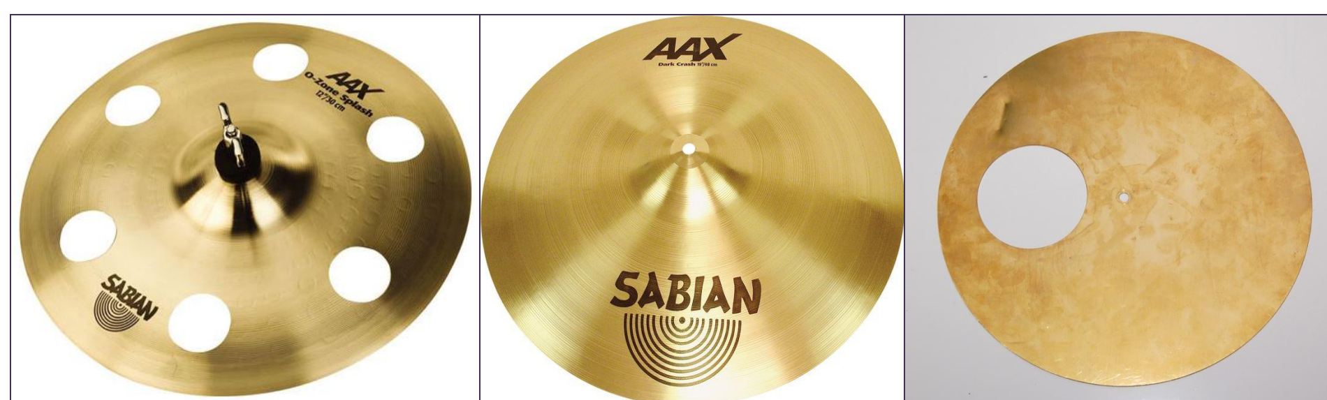
Figure 1. Three of the instruments used in this study. From left to right is the Sabian AAX Ozone cymbal, the Sabian AAX crash cymbal, and the 10 inch brass disk with a 3" inch diameter hole cut in the Puget Sound shop.
