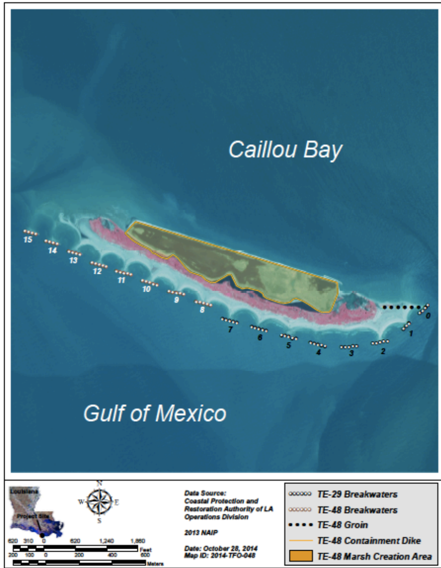
Figure 4: Design of the TE-29 breakwaters and TE-48 breakwaters and marsh creation area (source: Coastal Protection and Restoration Authority of LA, Operations Division.)
