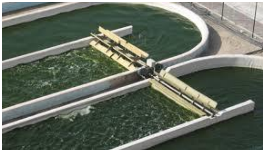
Figure 4. High-rate algal pond with a paddlewheel (Chinnaswamy, 2013).
