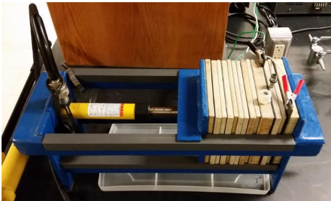
Figure 13. Electrochemical batch reactor (Simosa, 2016).
