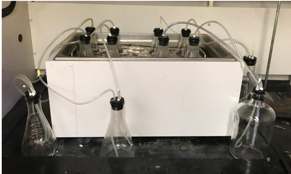
Figure 28. Experimental set-up of anaerobic digestion experiment.
