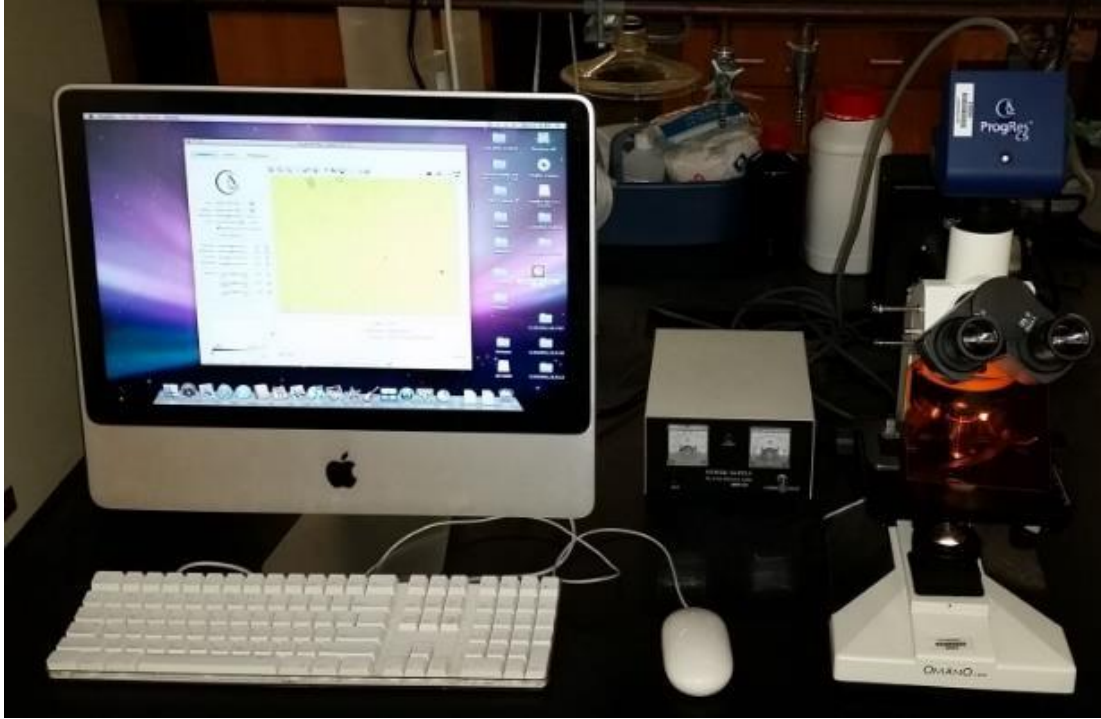
Figure 20. OMANO compound microscope assembled with a Jenoptik camera connected to a monitor (Simosa, 2016).
