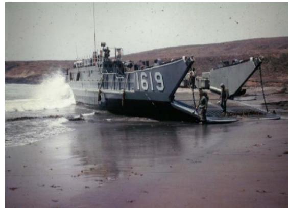
Figure 2. LCU-1619 broached while offloading tanks on San Clemente Island, CA. Surf lifted and pounded the hull on a large rock during the rising tide. (1964 picture courtesy of NavSource Naval History).
