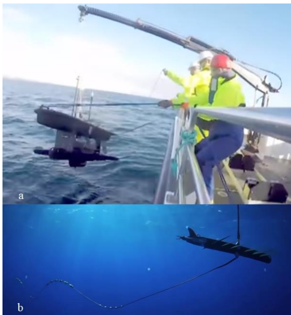
Figure 3. Liquid Robotics Wave Gliders operated 24/7 for 13 days during Exercise Unmanned Warrior. (a) Deployment of a Wave Glider on September 19, 2016. (b) The platform operated in seas of up to 21 feet and was outfitted with temperature, salinity, and acoustic sensors to support anti-submarine warfare missions in the North Sea. (Courtesy of Liquid Robotics).
