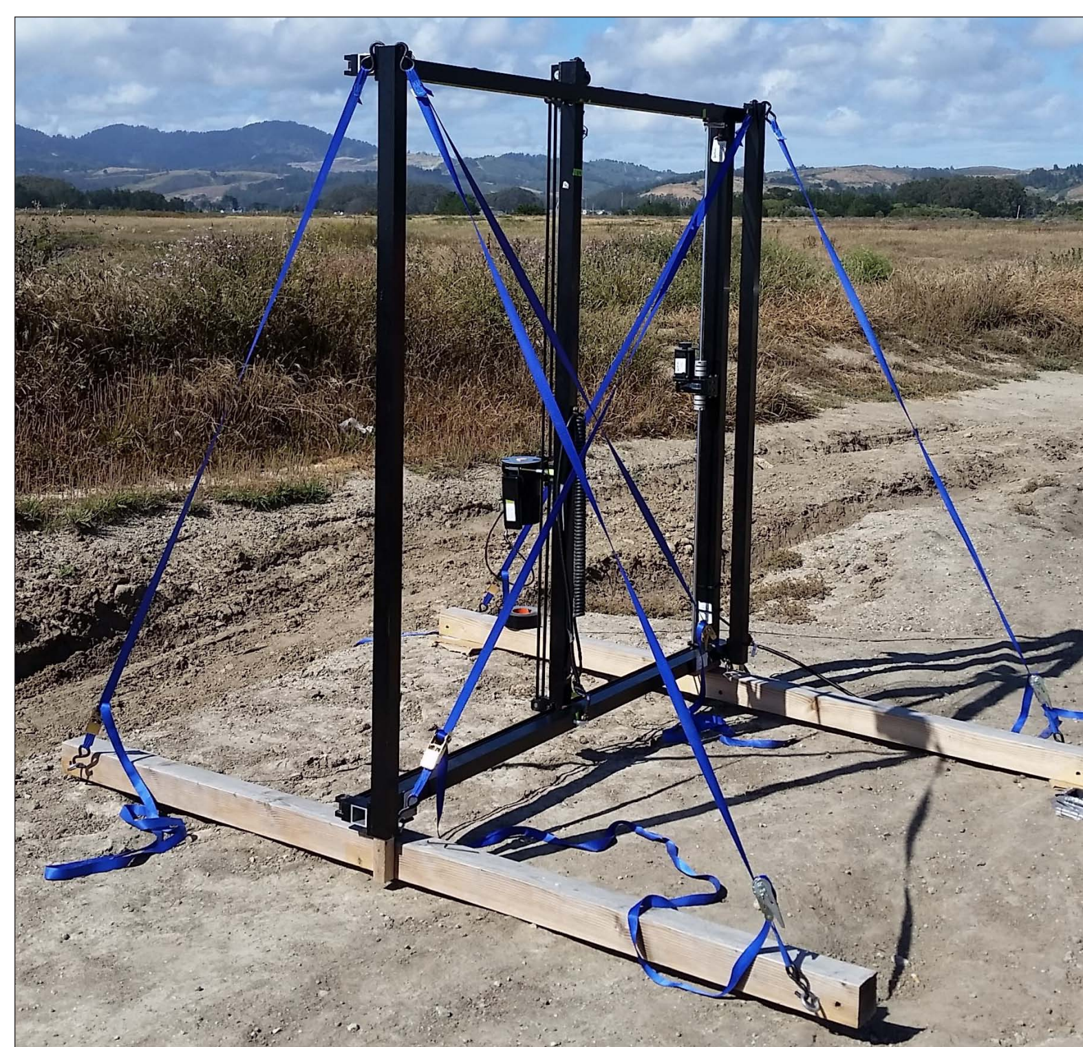
A custom-built 2-dimensional wave validation stand features two orthogonal arms and a programmable motion controller.
