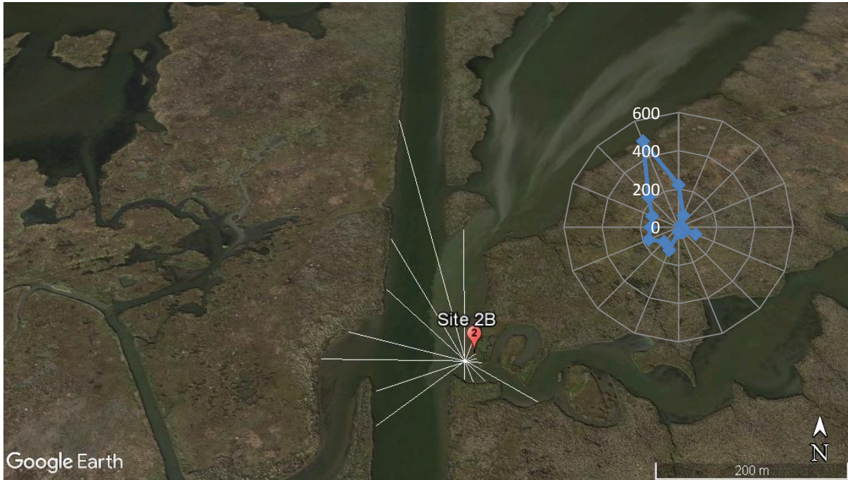
Figure 49. This image depicts Fetch distances and directions as they relate to the mouth of the inlet located at site 2B. Distance (in meters) from the center of the inlet mouth to the nearest shoreline is depicted as the blue line in the inset graph (2016 image from Google Earth).
