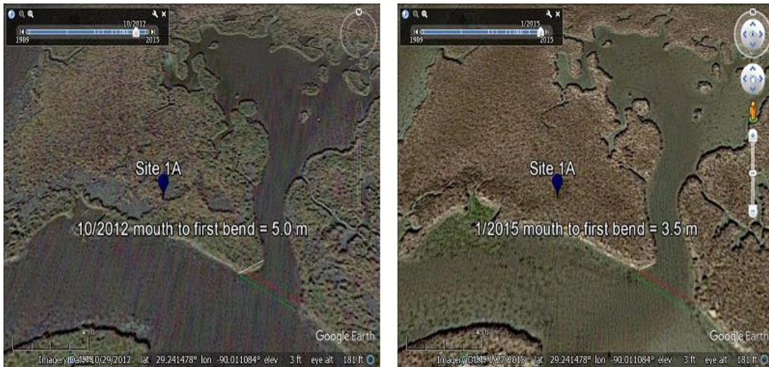
Figure 18. Image shows the narrowing of inlet due to shoreline retreat. As the shoreline adjacent to the mouth of the inlet eroded, narrower sections of inlet were exposed resulting in decreasing erosion measurements (2016 image from Google Earth).
