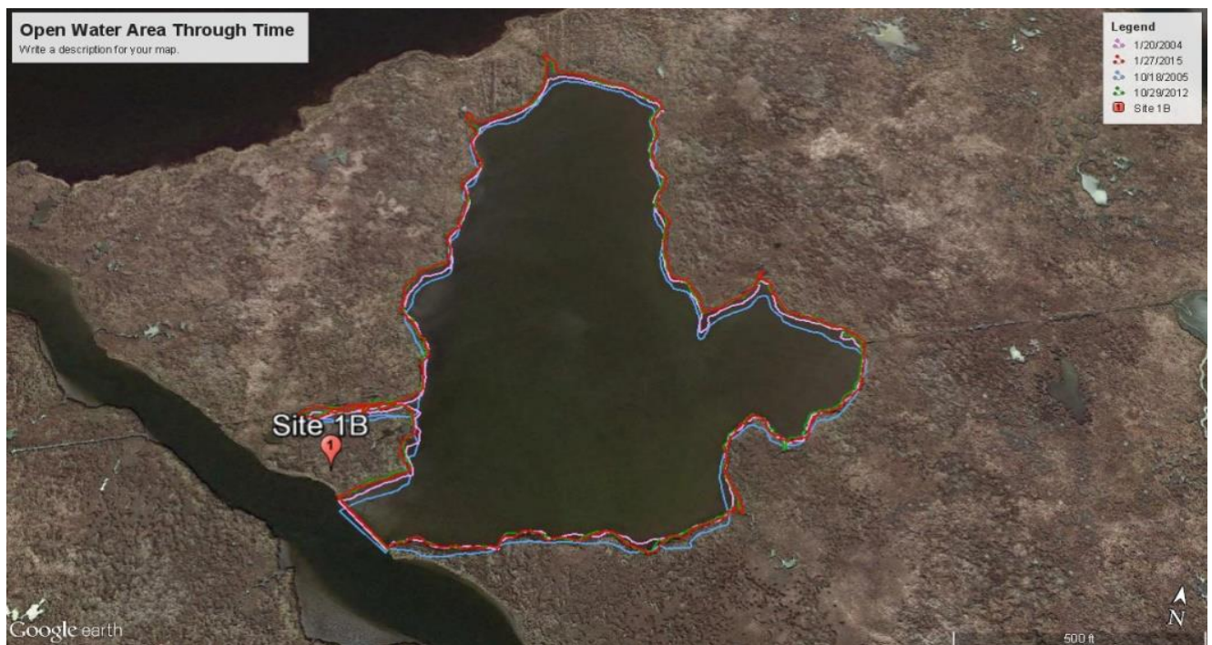
Figure 7. this image shows area measurements from the different image dates. Viewing measurements together demonstrates erosion of shorelines and channel inlet changes through time (2016 image from Google Earth).
