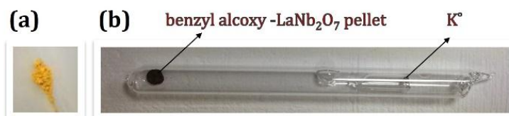
Figure B- 9: (a) sharp yellow BA-LN prior to intercalation, and (b) post-reaction picture of BA-LN pellet exposed to \text{K}^+ vapor under vacuum.
