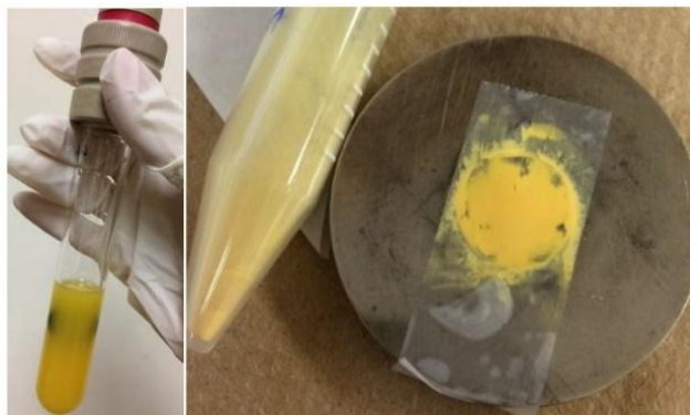
Figure B- 5: Sharp yellow color of as-synthesized benzyl alcoxy-LaNb 2 O 7 .
