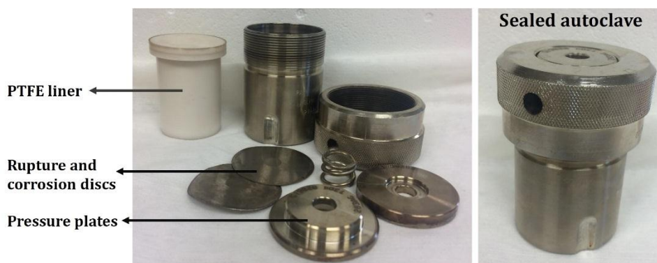
Figure 1-9: PTFE-lined cylinder and parts of a typical autoclave (left) and a sealed autoclave (right).
