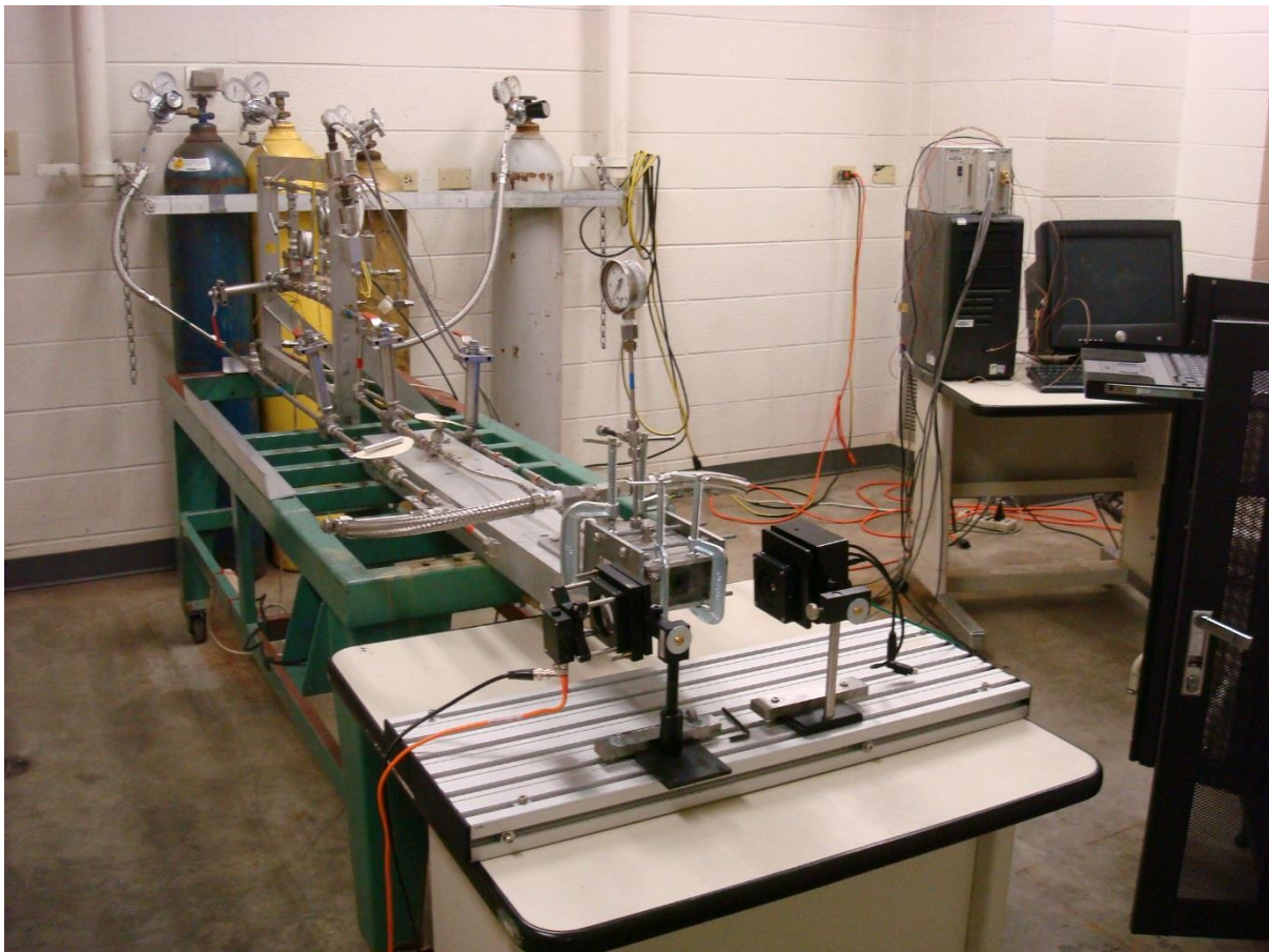
Figure 4. LPRM Test Stand, Gas Supplies and DAQ System
