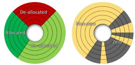
*Figure 2.3. Left portion: data representation from the filesystem's perspective. Right portion: raw data representation.*
