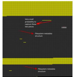
Figure 3.12. The chunk map produced by the allocationbased strategy for a 500GB disk without valid filesystems on it.
