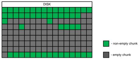
Figure 2.1. A disk represented as a set of fixed size chunks.
