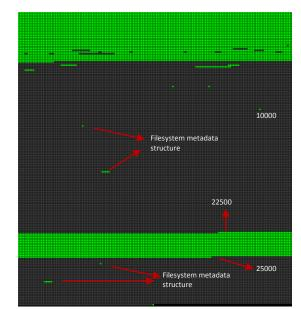
Figure 3.4. The ground truth chunk map for the 500GB disk with four NTFS filesystems.
