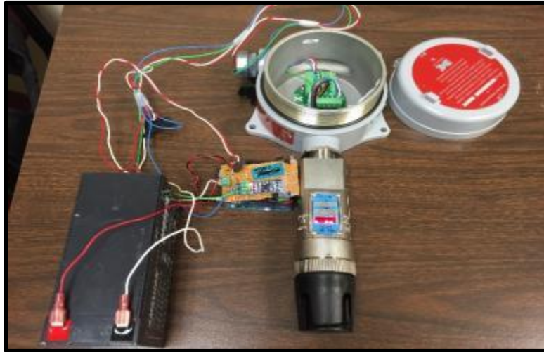
Figure 10: Arduino setup connected to sensor
