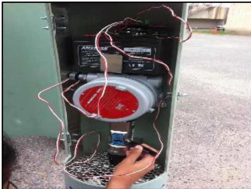
Figure 11: Housing with entire Arduino setup, sensor, and a battery
