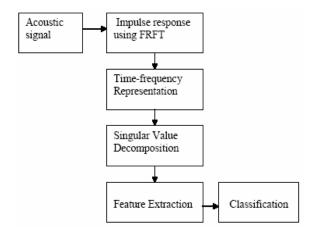
Fig. 1. Processing system for classification of return echoes.
