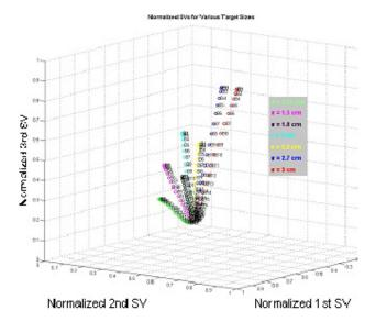
Fig. 4. Singular values of the Wigner distribution of targets of seven different diameters.
