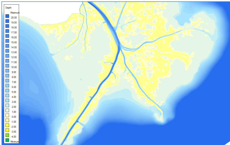
Figure 7-2 Detail of grid bathymetry in the birdfoot delta
