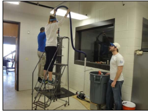
Figure 4.8- Mixing container (left) and pumping slurry into the column (right)
