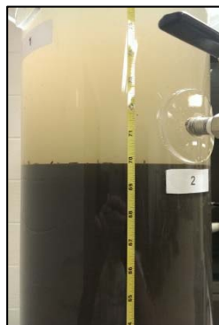
Figure 4.9- Sampling Protocol: Solid water interface (left) and sample extraction using needle (right)
