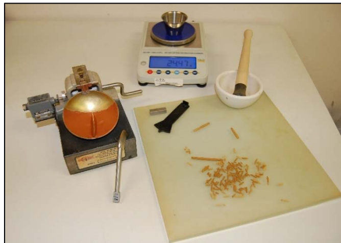
Figure 4.2- Atterberg Limit Equipment
