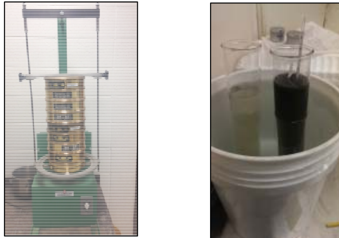
Figure 4.3- Equipment used in Sieve Analysis (left) and Hydrometer Analysis (right)
