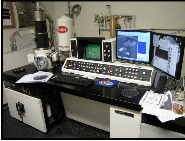
Figure 6 Amray 1820 SEM used for sample evaluation with Back Scattered Electron (BSE) images and creating X-ray maps.
