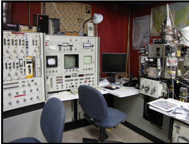
Figure 7 Quantitative chemical analyses of samples were obtained using an ARL-SEM electron microprobe.
