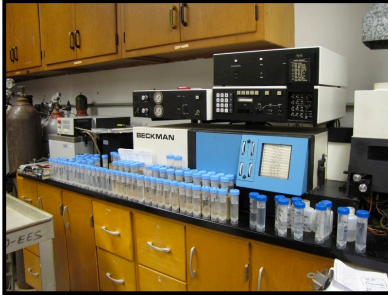
Figure 8 A Beckman Spectraspan V, Direct-Coupled Plasma (DCP) spectrophotometer used to determine concentrations of trace elements.
