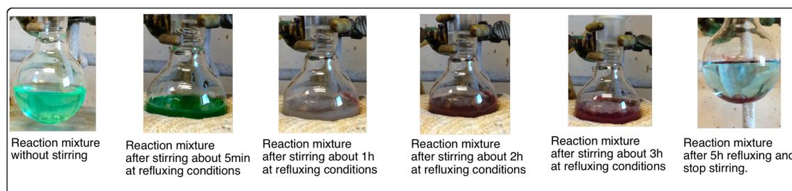
**Figure 5.8** Reduction of  $\text{CuSO}_4 \cdot \text{H}_2\text{O}$  in DMF
