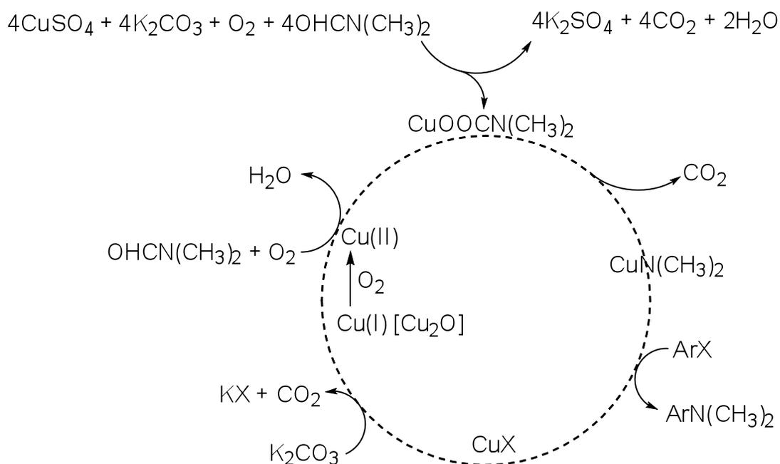
**Figure 4.2:** Proposed mechanism for  $\text{CuSO}_4 \cdot 5\text{H}_2\text{O}$  catalyzed coupling of aryl halides with N,N-dimethyl formamide (DMF).
