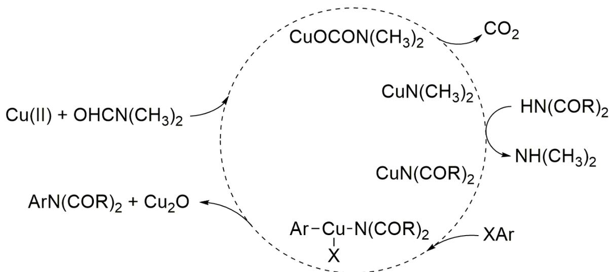
**Figure 5.9** Proposed catalytic cycle for coupling of cyclic imides with aryl halides
