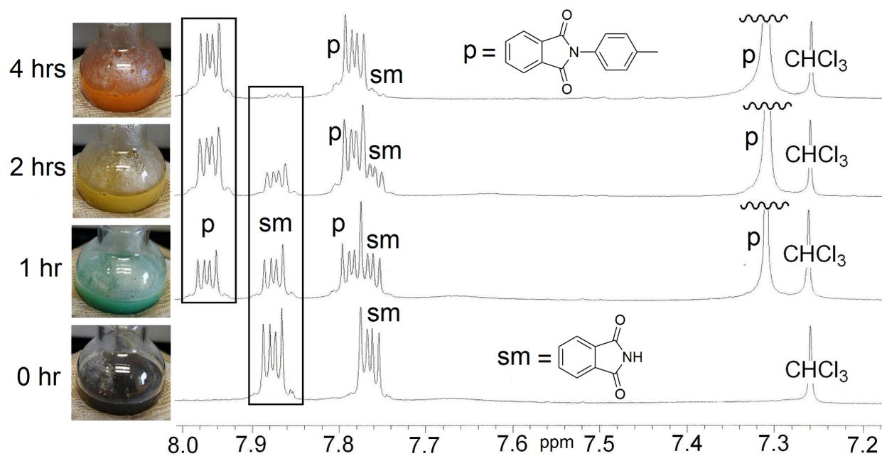
**Figure 5.6** Visual and <sup>1</sup>H-NMR reaction monitoring of DMF refluxing suspension of potassium phthalimide, *p*-bromotoluene, and copper (II) sulfate pentahydrate
