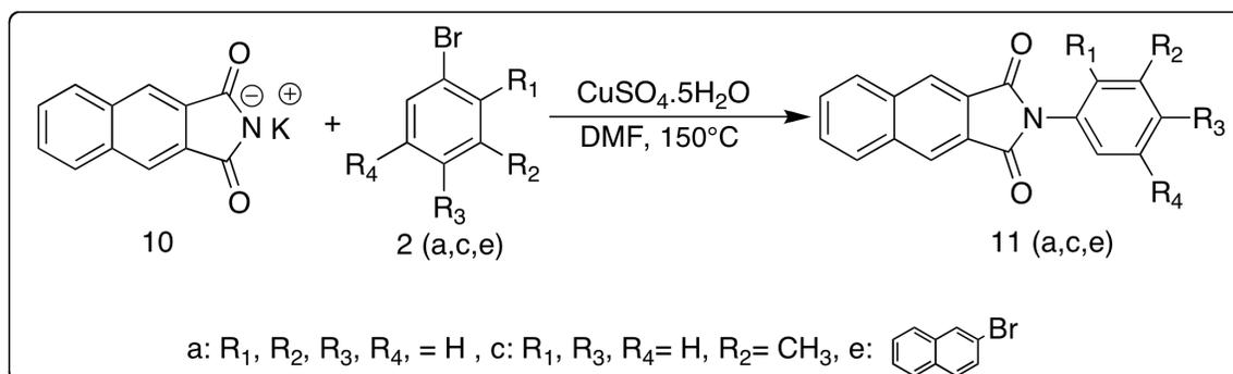
**Scheme 5.8** Potassium-2,3-Naphthalimide coupling with aromatic halides.
