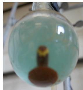
(f) After refluxing in DMF for 4 h and left at R.T for 10 Min
