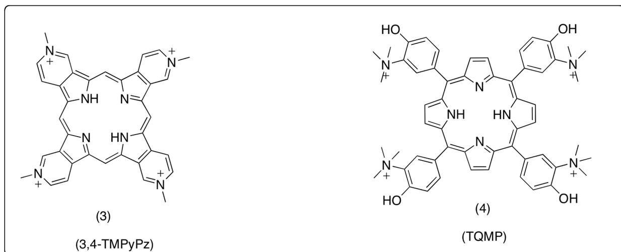
**Figure 1.17** Structures of 3,4-TMPyPz and TQMP
