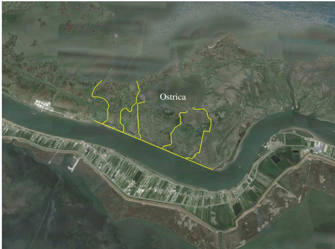
Figure 5-5: Ostrica outlets marked on Google Earth image (RM 22 to RM 26).
