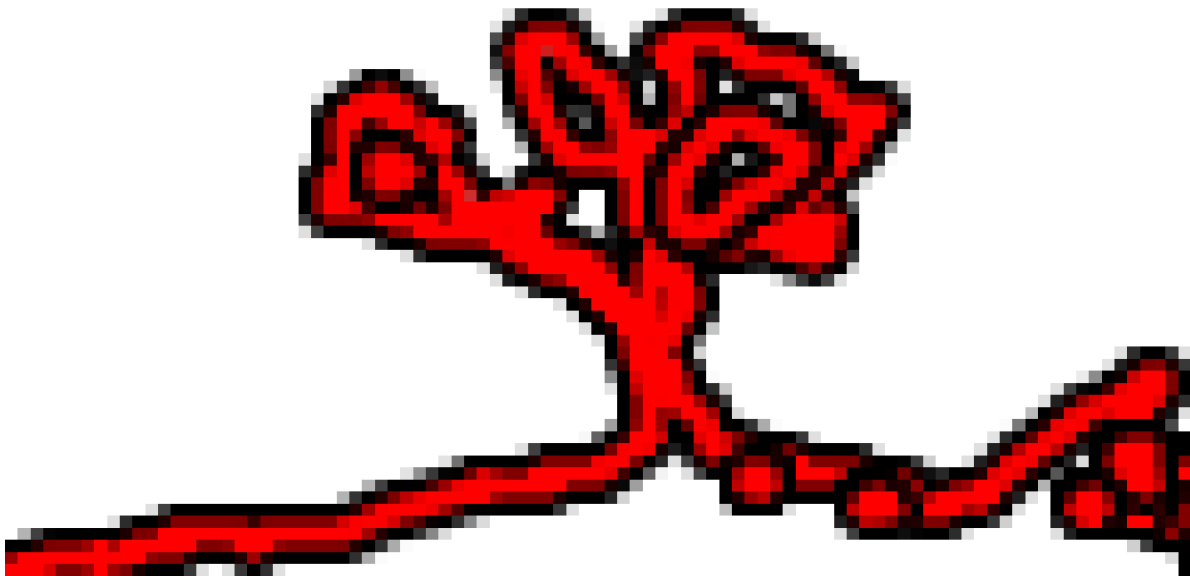
Figure 8. When zooming into the static image from Figure 7, Pearl Harbor shorelines become thickened and blurred. This shows that precision has been increased past the accuracy in the original image.
