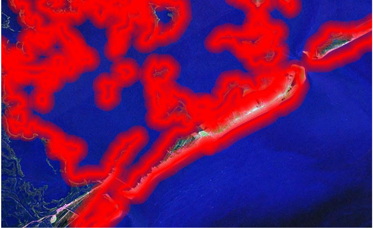
Figure 14. “Transparency Gradient”: Renders a shoreline width buffer that is a solid color at the center and gradually fades to transparent at the edges. Indicates decreasing certainty towards the edges.
