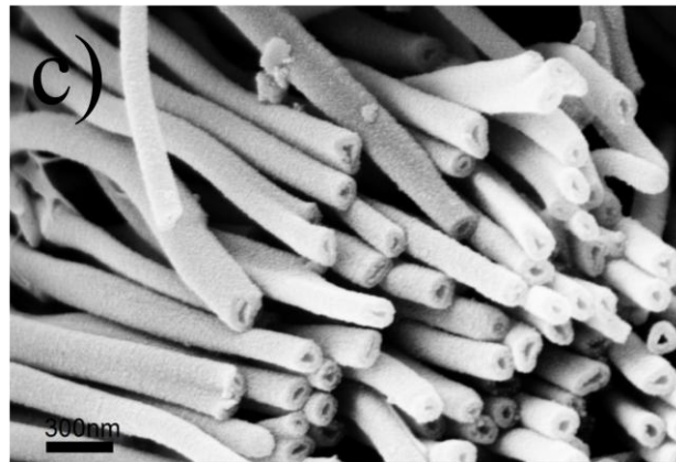
Figure 4.3. FE-SEM images of the BaTiO 3 nanotubular architectures a) confined in the AAO template, b) partially exposed and c) free standing
