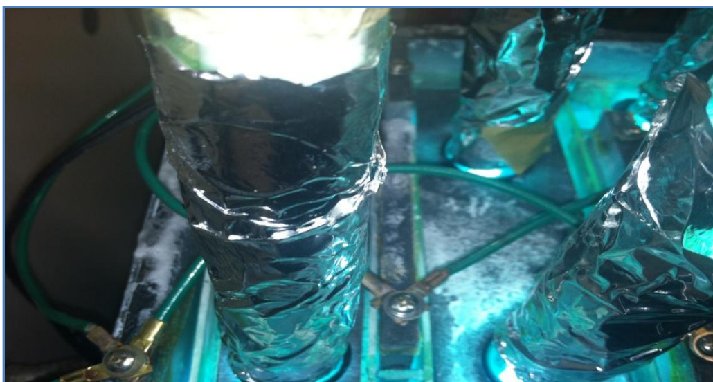
Figure 14. Photocatalytic operation of 3 cell reactor
