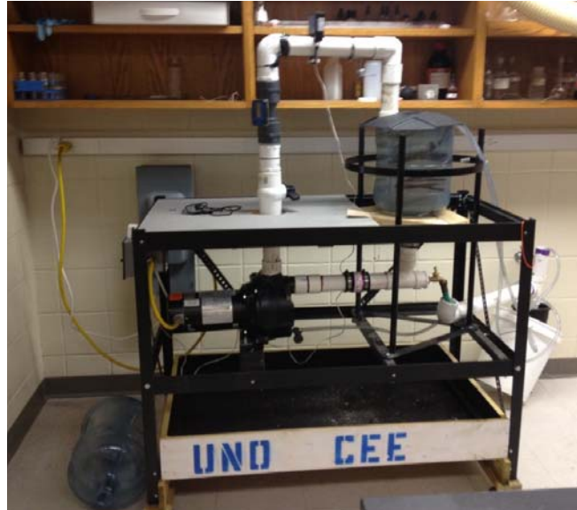
Figure 15: Experimental Design with basin, pump, flowmeter, and unit in place. The design was altered to accommodate temperature changes associated with longer runtimes
