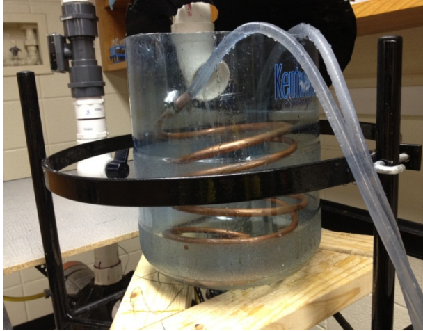
Figure 13: Heat exchanger to regulate temperature
