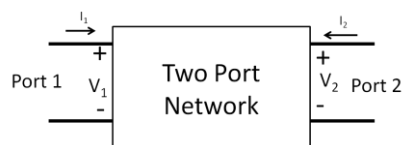
Fig3.2d: A general two port network
